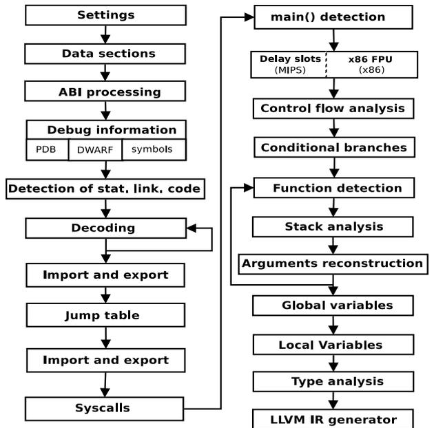
Figure 2: The architecture of *decfront*.
