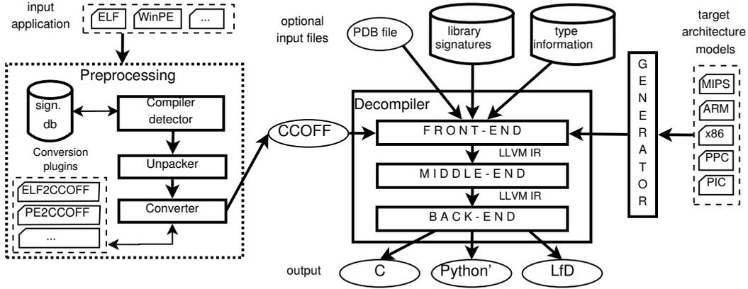
Figure 1: The concept of the retargetable decompiler.
