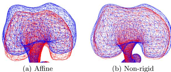
Figure 4: Comparison of two levels of registration of source mesh (red) to target mesh (blue). Bottom head of Femur bone.
