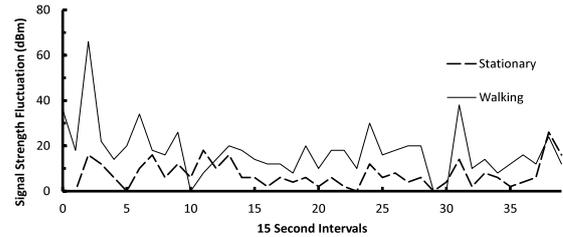
Figure 1: GSM signal strength fluctuation.
