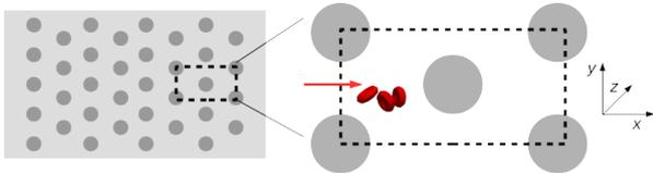
**Figure 7:** On the left is scheme of periodic array of obstacles and selected simulation box. On the right is scheme of simulation box, arrow shows the direction of flow, black dotted lines show boundary of box with periodic boundary condition.
