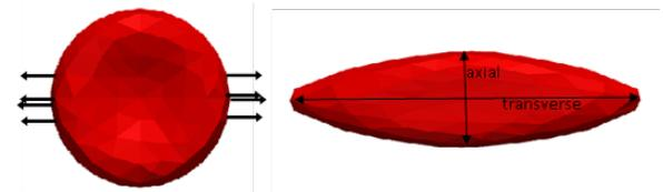
**Figure 5:** On the left, we see the beginning of simulation, the cell is stretched by applying force at several nodes on surface (black arrows). On the right is final stage of simulation - relaxed state, we measured transversal and axial diameter.
