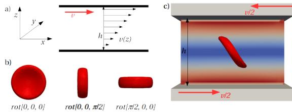
**Figure 3:** In a) is scheme of Couette flow in channel, where top plate is moving with velocity  $v$  and bottom plate is not moving. Inside the channel, the flow velocity is function of height  $z$ . In b) are shown selected rotation of RBC and their marks. In c) is simulation scheme of RBC in shear flow. Both plates are moving in opposite direction with velocity  $v/2$ . The color of fluid corresponds with its velocity from maximum near the plate (red) to minimum in the middle (blue).
