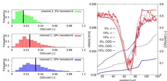
**Figure 11: On the left histograms for channel 1, hematocrit 5% (green), 10% (red) and 15% (blue). On  $x$ -axis are achieved values  $CDG(cell)$ . On  $y$ -axis is frequency of cells from given interval, normalized to total cell number from the set of simulations. On the right is dependency of cell velocity on position in channel for chosen cell for hematocrit 5%, 10% a 15% - red lines. With blue lines are depicted dependency of  $CDG(cell)$  for chosen cell on position in channel.**
