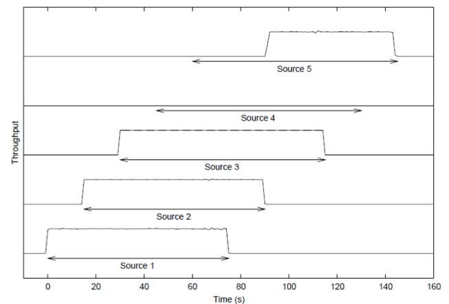
**Figure 3: Throughput of data flows with admission control.**
