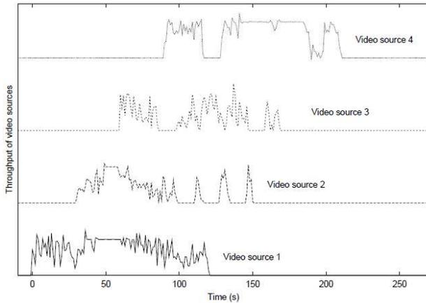
**Figure 4: Throughput of data flows in Video priority class without admission control.**
