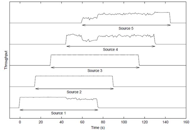
**Figure 2: Throughput of data flows without admission control.**
