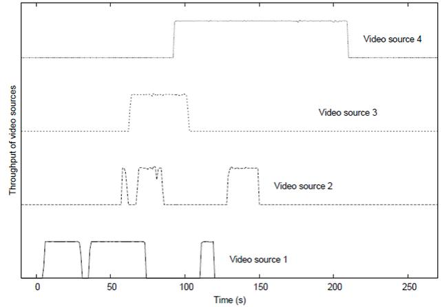
**Figure 5: Throughput of data flows in Video priority class with admission control.**
