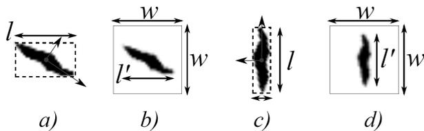
**Figure 2: Image normalization.** a) source image with particle bounding box and major and minor axes, b) image normalized to size  $w$  without rotation, c) rotation of the original image with new bounding box and d) image normalized with rotation.
