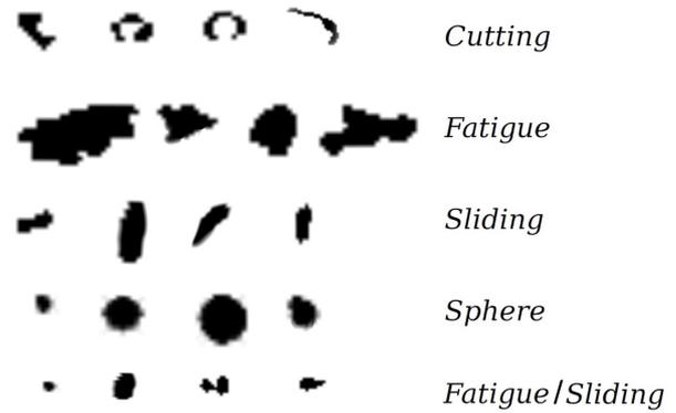
**Figure 1: Classes of particles with typical representatives**
