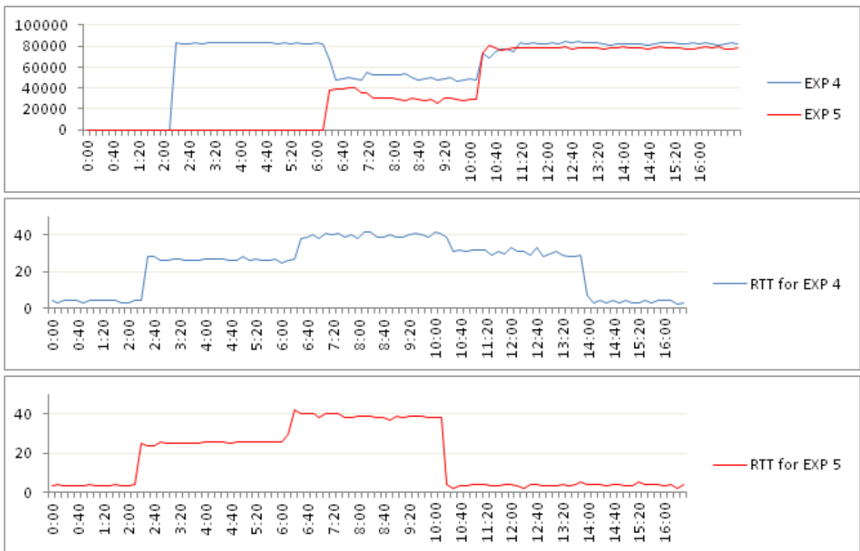
Figure 11: Experiment 2 - measured throughput in kb/s (top figure) round-trip time for EXP=4 traffic in ms (middle figure) and round-trip time for EXP=5 traffic in ms (bottom figure)
