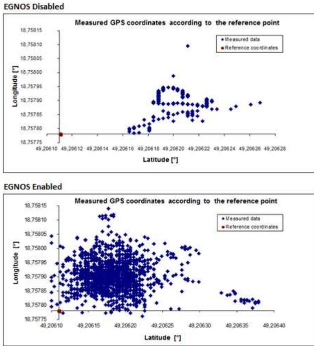
Figure 13: Measured coordinates with EGNOS support disabled/enabled.
