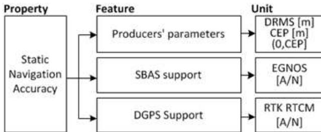
Figure 15: Static Navigation Accuracy Features of GNSS receivers.
