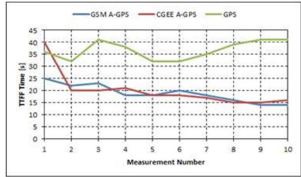
Figure 8: Comparison of acquisition times between GSM A-GPS, CGEE A-GPS and common GPS receiver in the measurement taken in 20th November 2012.
