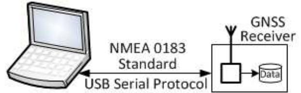
**Figure 12:** Control of GNSS receiver through NMEA 0183 via USB.
