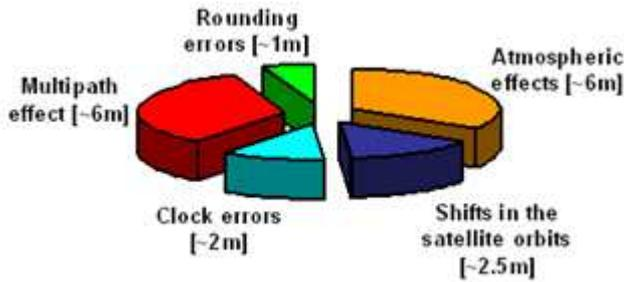
Figure 2: Graphical interpretation of the GNSS error sources and the size of error that they cause.
