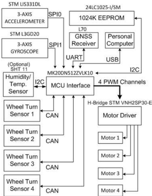
Figure 24: The concept of the experimental inertial navigation system.
