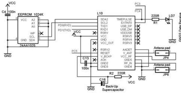
Figure 7: Simplified schematic of CGEE A-GPS system based on ATMega8.
