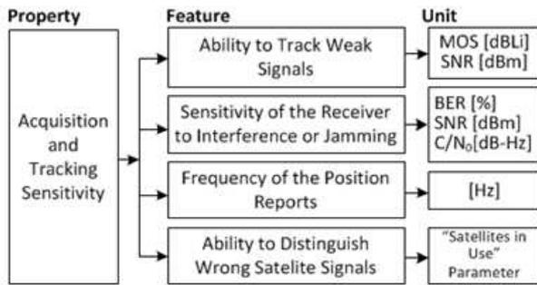
Figure 5: Acquisition and Tracking Sensitivity Features of GNSS receivers.
