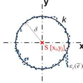
**Figure 1: Circle interpretation of the static 2D localization function.**
