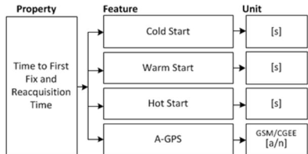
Figure 9: TTFF and Reacquisition Time Features of GNSS receivers.
