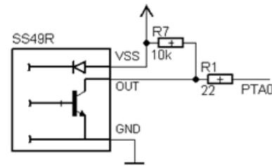
**Figure 22: Hall Effect sensor design / simplified.**
